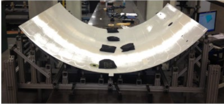
Figure 1 – Aerospace panel achieves functional shape under permissible loads (black sandbags) [4].
