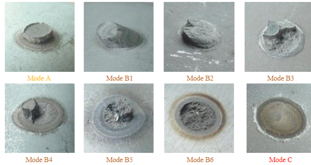
FIGURE 4 – Modes de rupture des PSR [1]
